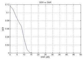
Fig: 4(d). SER of AWGN Channel
