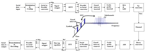
Fig: 1. Block Diagram of OFDM System
