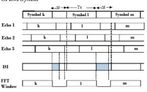
Fig: 3 (a). Combining ISI using a Guard Period [1]
