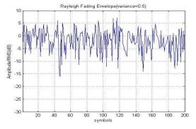
Fig: 4(i). Rayleigh Multipath Channel with AWGN Fading Envelope
