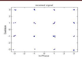
Fig: 4(b). Received 16-QAM Constellation Diagram
