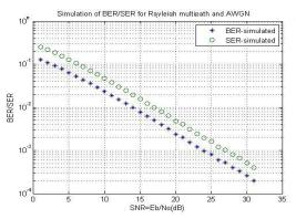
Fig: 4(h). BER and SER of Rayleigh Multipath Channel with AWGN Channel
