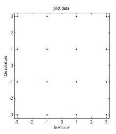
Fig: 4(a). Transmitted 16-QAM Constellation Diagram
